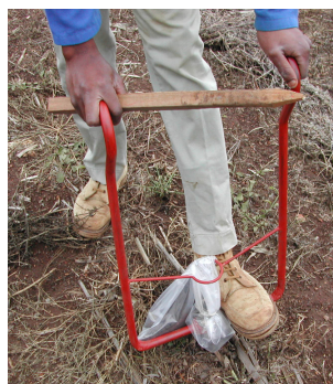
Figure 7 & 8: These show the beater soil sampler being thrust into the soil and the forcing of the subsample (core) from the sampling bit into the plastic bag.
