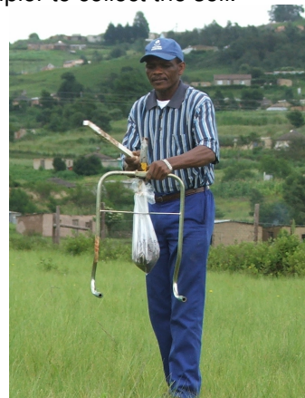
Figure 2: Using a beater soil sampler with a 15 cm bit to take a soil sample.
