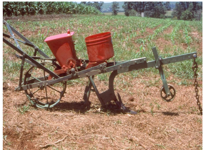
Figure 6: An animal-drawn single-row no-till planter without coulter attached.
