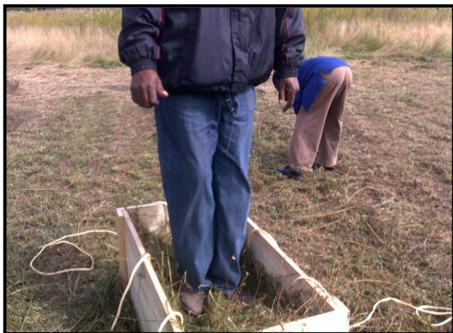
FIGURE 3: Compacting the material when making bale
