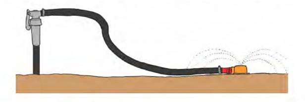
WHEN THE PIPELET IS DISCONNECTED, THE HYDRANT AUTOMATICALLY CLOSES THE WATER OFF.
