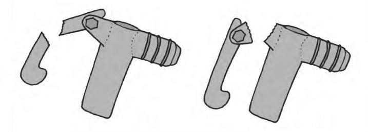
IF THE HYDRANT LEAKS, IT MUST BE UNSCREWED FROM THE STANDPIPE AND REPLACED.
