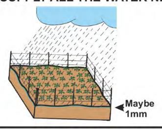
IRRIGATION IS USED TO SUPPLEMENT THE RAIN WATER. VEGETABLE CROPS NEED 5mm OF WATER EVERY DAY.
