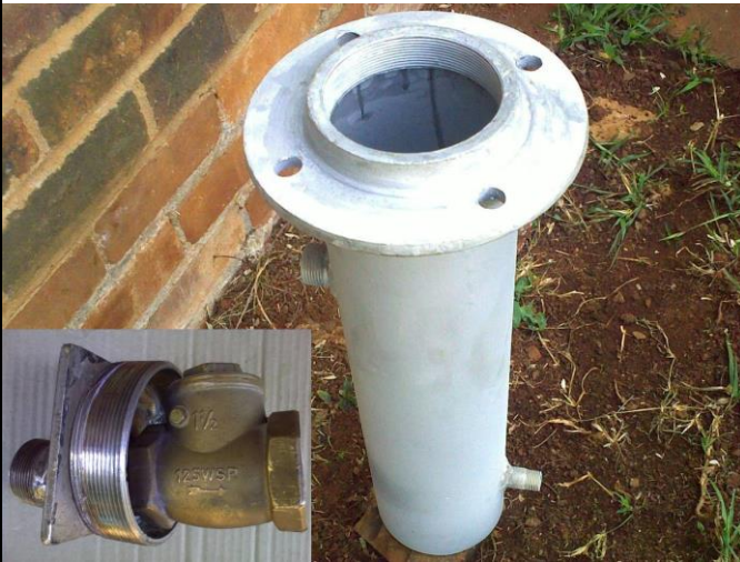
Fig. 1.3 Ram pump steel pressure vessel (main view) showing threaded opening on top, output nipple (left side) and a pressure-release nipple (lower right side). The Inset lower left shows the fitting with attached non-return valve that screwed into its opening.
