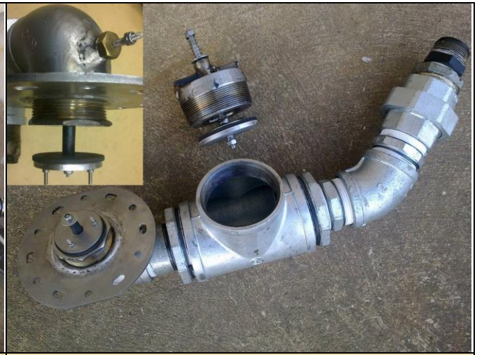
Fig. 7.6 The operating valves of the ram pump disconnected from the pressure vessel. The top left inset shows the flanged elbow with snifter valve and non-return valve (in open position).
