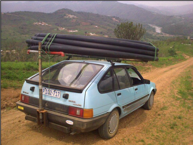
Fig. 2.1 My own Toyota Avante fitted with a tow bar strut that connected to a cross member on the roof rack for transport of 100m of HDPE 50 mm piping needed for the ram pump site. Mkomazi river in background.
