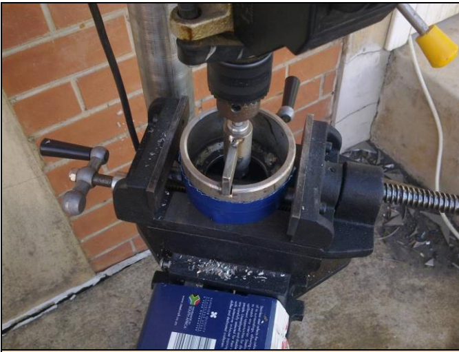
Fig. 7.5 Mounting of the central guide pipe of the impulse valve prior to welding it to the body of the impulse valve. Alignment done using a drill press.
