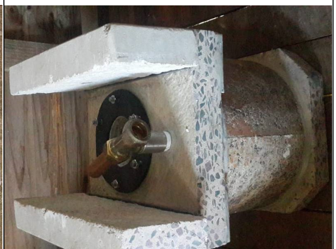
Fig. 7.4 Underside of completed pressure vessel with ram pump operating valves disconnected from it.
