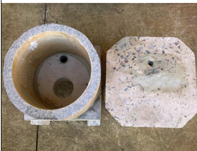
Fig. 7.3 Completed pressure vessel prior to epoxying the top end on.
