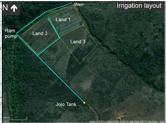
Fig. 6.2 A Google maps satellite photo of the Vulamehlo ram pump installation site with location of irrigation system and land units superimposed.
