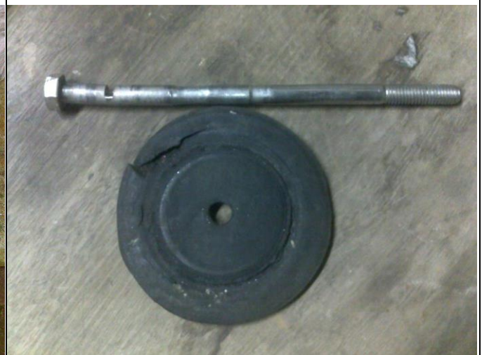
Fig. 1.6 Bolt axis of impulse valve (upper) showing severe abrasion after several months of operation and lower seal showing wear and a tear.
