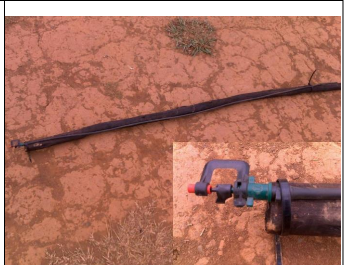
Fig. 6.4 Microjet sprinklers were made up and attached to creosote poles for installation according to the proposed low pressure sprinkler system (Fig. 6.3) but these were not installed before the project ended.
