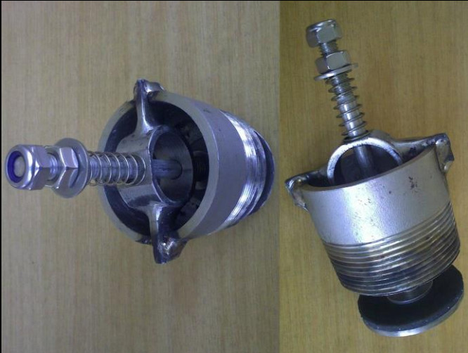
Fig 1.1 Impulse valve of stainless steel. The body was a 3 inch BSP barrel nipple cut in half with a disk welded to the bottom end. A cut pipe segment with flange was welded to the top as a guide for the axis of the valve with seal on its end.
