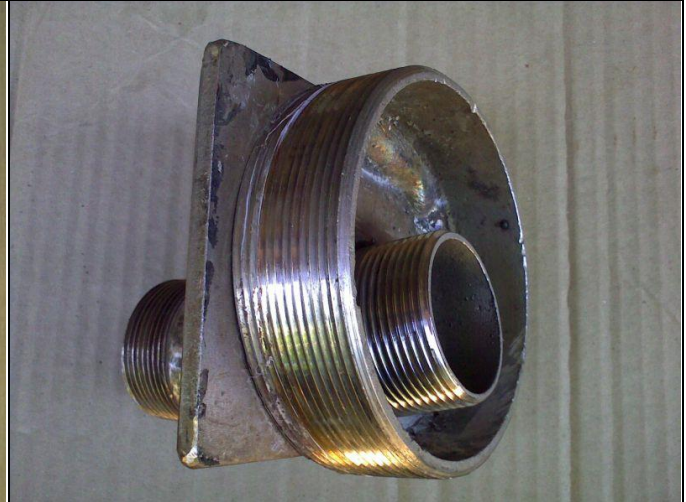
Fig. 1.2 A stainless fitting made to screw into the pressure chamber with the outer nipple (at left) connecting to a T in which the impulse valve fitted, and the inner nipple (at right) connecting to a flap-type non-return valve.
