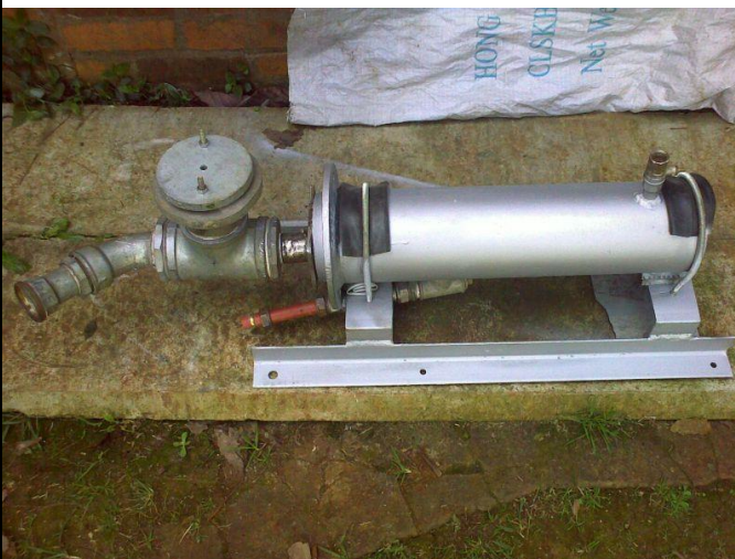
Fig 1.5 Assembled ram pump. Initially the impulse valve was fitted with disk-weights for control which were removed later as it operated better without them.
